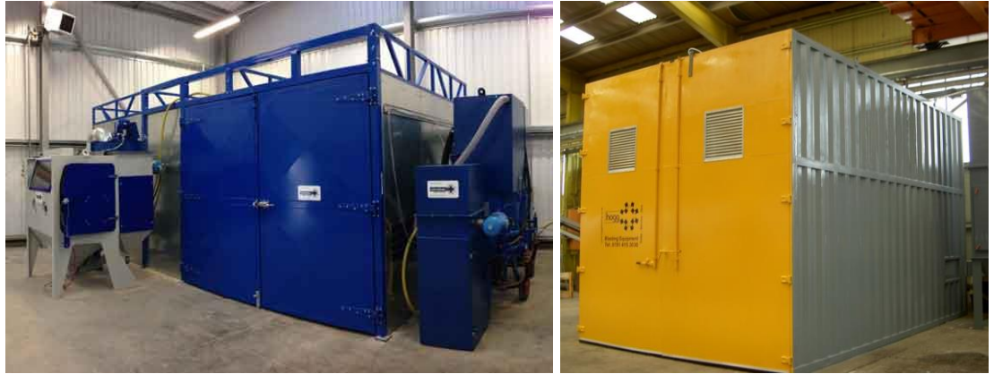
Modular Blast Room and Cabinet (left) and Containerised Blast Room (right)
